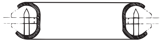
Completely and correctly closed Inox Ring
